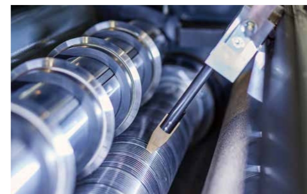
Positioning aid Time saving and precise alignment for bottom knives and grooved bushes.
