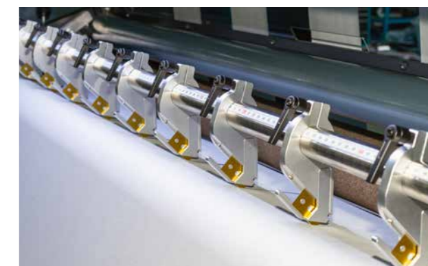
Razor blade cut Reasonable and good. Optionally as groove or mirror cut.
