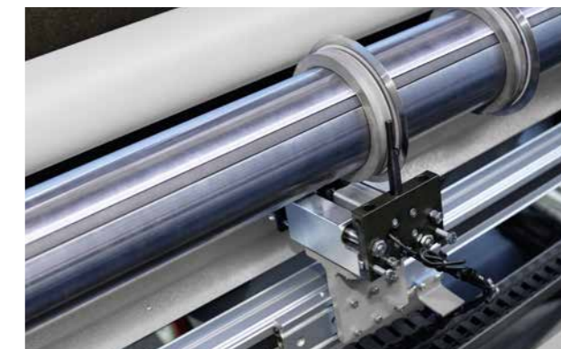
Automatic knife positioning For repeatable exact slitting positions and set-up time reduction.
